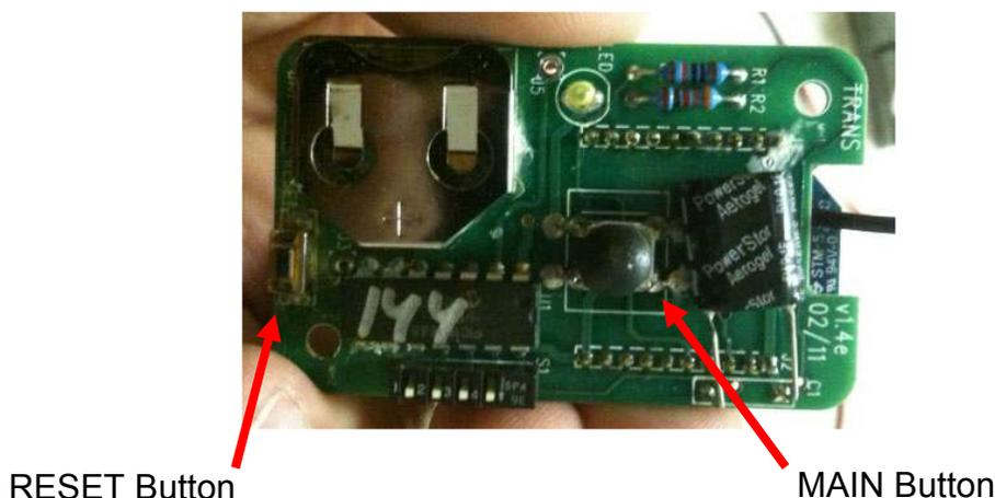
1. Open the remote control case and remove the circuit board.
