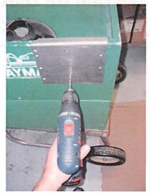
3. Drill a ½ inch hole for the wire-kit to go through as marked below. This will let the wire-kit connect to the new receiver that will be mounted up in the front top of the ball machine.
