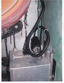
It's important to make sure that the cable is secured so that it cannot get loose and touch the pitching wheels or chain. If you have, tie the wire in a coil in order to remove any slack or try distributing the slack along the wire-kit from the control box connection around the top front as it heads towards the new receiver.
