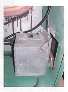
9. Plug the new wire-kit into the control box and tie up any loose wires.
